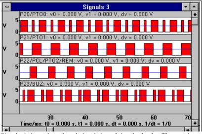
Signal windows show the relative timing of signals clearly. They can be scrolled backwards to see the past changes. The amount of past detail that is stored depends on the buffer size. For more information about using plot records see the later section.
