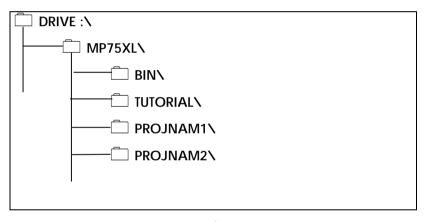
The BIN sub-directory contains all the executable files, with the exception of the build tool executables. Note that the tutorial files are not required for the normal operation of Micropak 75XL.
