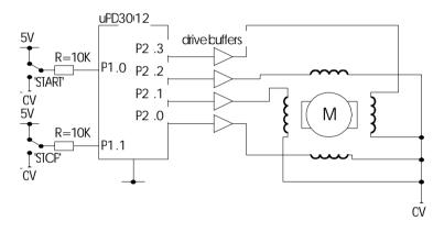
The simple stepper motor driver used as an example
